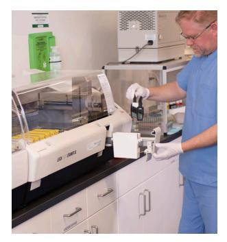
At the end of the staining run, the stainer may sound an alarm to alert the attending laboratory personnel to remove the slide rack from the stainer for subsequent coverslipping. Alternatively, some automated slide stainers are made to be coupled to a transfer station, which moves the slide rack from the stainer into an automated coverslipper. This equipment will be the subject of the next article. ABOUT THE AUTHOR: Clifford M. Chapman BS, MS, HTL (ASCP), QIHC
