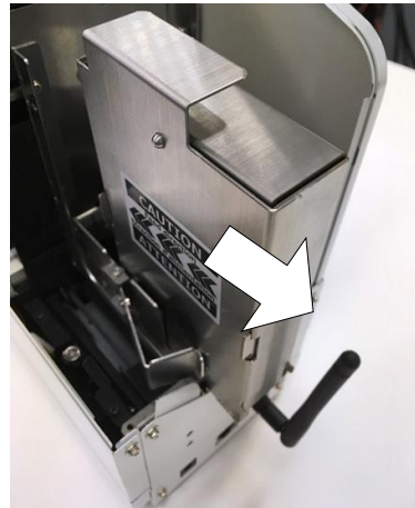
The guide opens. Pull out the magazine from rear side.
