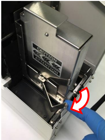
The guide opens. Pull out the magazine from rear side.
