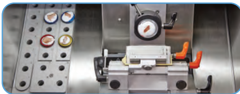
Peltier provides fast freezing (-55°C) for 4 stations (27 freezing stations total)
